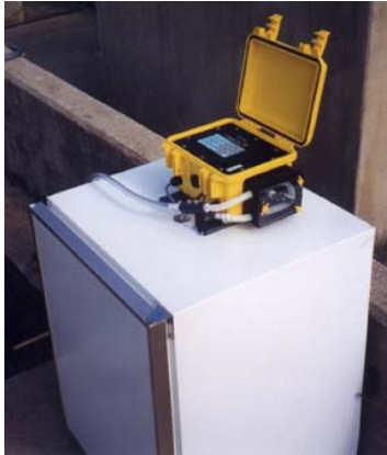
YB Sampler with Standard Refrigerator
