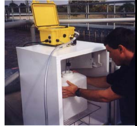
YB Sampler with Single Bottle
