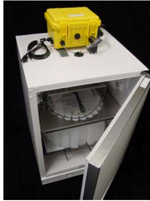
YB Sampler with Multi-bottle Option
