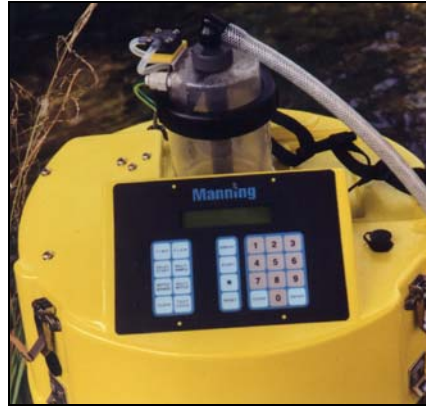
Manning VST Sampler Control Panel
